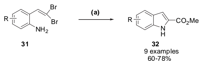
Scheme 14. Reagents and conditions: (a) 31 (1.0 mmol), \text{PdCl}_2(\text{PPh}_3)_2 (5 mol %), \text{PPh}_3 (10 ml); DIPEA (2.0 mol equiv), CO (10 atm), THF/MeOH (1:1 v/v, 8 ml), 110 °C, 20 h.
